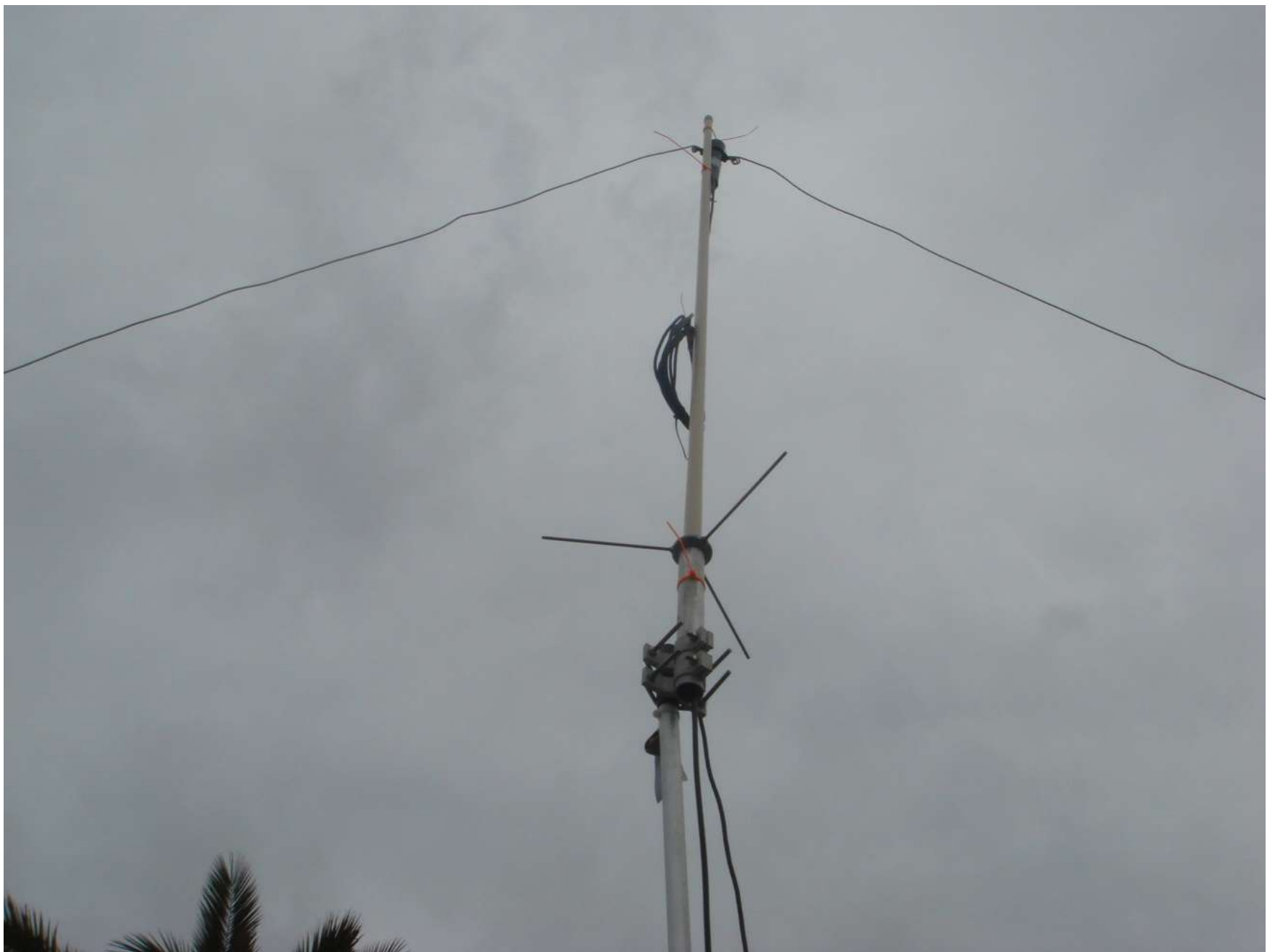
Our 2M/440 antenna with a 15M dipole on top
