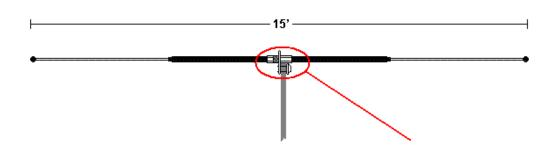
THE TWO HamStick DIPOLES ARE ATTACHED TO A "T" BRACKET MOUNT WITH QUICK DISCONNECT FITTINGS FOR CHANGING OUT THE RADIAL ELEMENTS FOR DIFFERENT BANDS. THE "T" BRACKET'S U-BOLTS ACCEPT UP TO A TWO-INCH MAST.
