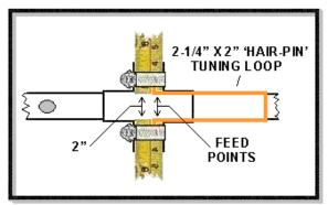
ALL ELEMENTS ARE MADE FROM LENGTHS OF ONE-INCH STEEL TAPE MEASURE.
