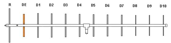
Spacing between elements is 5-1/2" Center-Point to Center-Point
