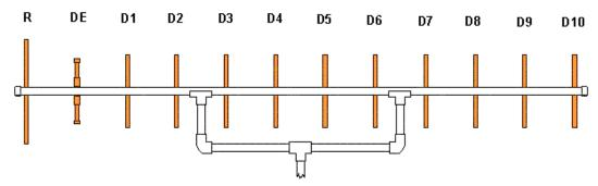
Spacing between elements is 5-1/2" Center-Point to Center-Point
