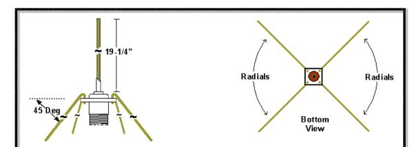
ASSEMBLE TWO 1/4 ~ GROUND PLANES USING SO 239 CHASSIS MOUNTS AND 1/8" BRASS ROD. FOR THE GROUND RADIALS, CUT EIGHT LENGTHS OF 1/8" BRASS ROD TO 18-1/2". BEND THE LAST 1/2" INTO A "J" SHAPE AND SOLDER EACH IN THE BOLT HOLES OF THE SO 239 CHASSIS MOUNT, AND BEND TO A 45° ANGLE. FOR THE RADIATING ELEMENTS, CUT TWO LENGTHS OF 1/8" BRASS ROD TO 19-1/4" AND SOLDER EACH TO THE CENTER POST OF THE SO 239 CHASSIS MOUNT.
