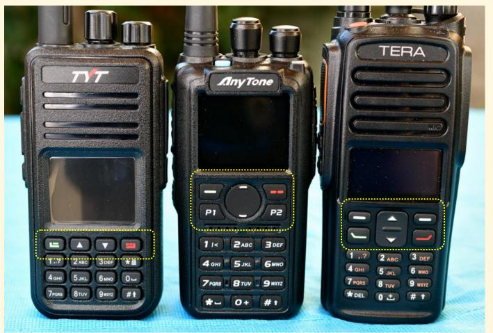
**Awkward:** Up/Down and menu selection keys difficult to use with thumb-only one-handed operation. May need to use both hands. Four-column keypad feels cramped . "Zero" button out of place, not at bottom of keypad like most radios.
