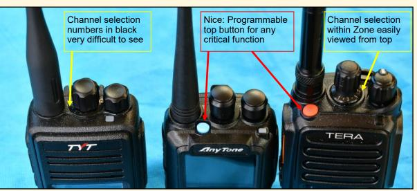
**Fair:** No programmable top button for emergency or scanning modes; hard to read channel selector (center) numbers in black on black. **Fair:** Has programmable top button but no channel selector markings; knobs feel slippery without ribs **Excellent:** Has programmable top button and highcontrast channel selector markings; great knobs
