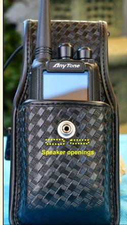
**Poor:** Display fully exposed to possible damage and speaker in center of radio is totally covered by holster...speaker mic needed with a holster.
