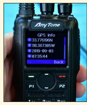
**Nice feature #1 on AnyTone 878UV:** Builtin GPS system works great but it's buried in the Menu options. Be advised: GPS screen only stays on for 10 seconds before reverting to home screen...if you haven't copied the coordinates by then you need to start all over through the Menus to reach the GPS.
