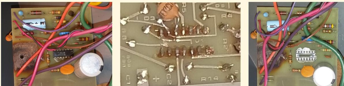
**Figure 1.** (left) Voltage regulator board with 14-pin LM723 integrated circuit shown prior to its removal; (middle) Solder side of IC prior to solder removal using flux-infused copper braid wicking technique; (right) Component side of board after installing IC socket for ease in replacing IC should it fail in the future. Note in left and right panels an area of PCB discoloration from overheating of (now removed) TIP29 driver transistor and heat sink. PHOTOS: JERRY KENDRICK, NG6R
