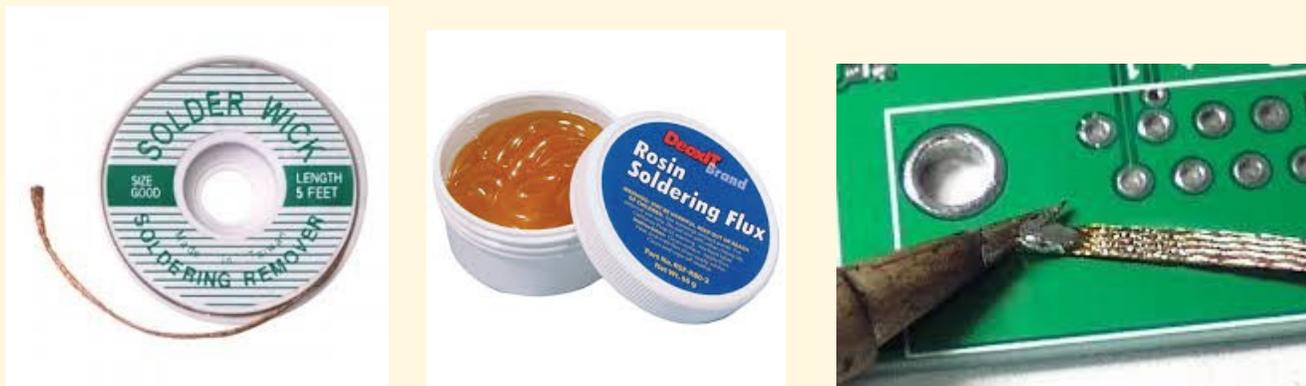
**Figure 3.** (left) Roll of fine-mesh copper braid, used to “wick” away melted solder; (center) Small container of rosin soldering flux into which the tip of the copper braid is dipped prior to each wicking attempt (very important!); (right) Hot soldering iron and braid tip are simultaneously placed onto the solder ball that is to be removed; note the flux that has soaked into the braid a few millimeters up from the tip of the braid.
