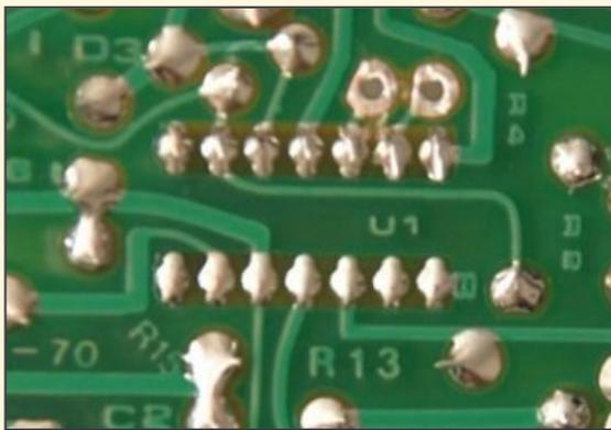
**Figure 1.** Solder side of Astron power supply voltage regulator board with 14-pin LM723 integrated circuit shown prior to removal
