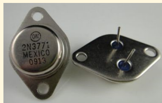
Figure 3. (left) Typical Astron PS voltage regulator PCB. Note the 14-pin LM723 plugged into its IC socket at the center of the board. (center) TIP29 transistor that drives the bases of the pass transistors and which can be seen attached to a heat sink at center left on the PCB. (right) Top and bottom views of 2N3771 series pass transistors; these are placed on heat sinks on the rear panel of each PS.
