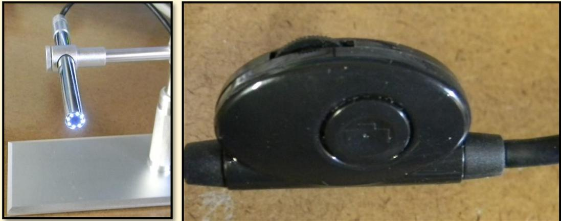
Figure 3. LED lights (*left photo*) and (*right photo*) in-line light intensity thumbwheel adjustment; snapshot pushbutton on side of control. PHOTOS: JERRY KENDRICK NG6R
