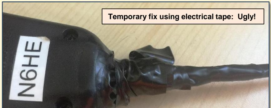
Temporary fix using electrical tape: Ugly!
