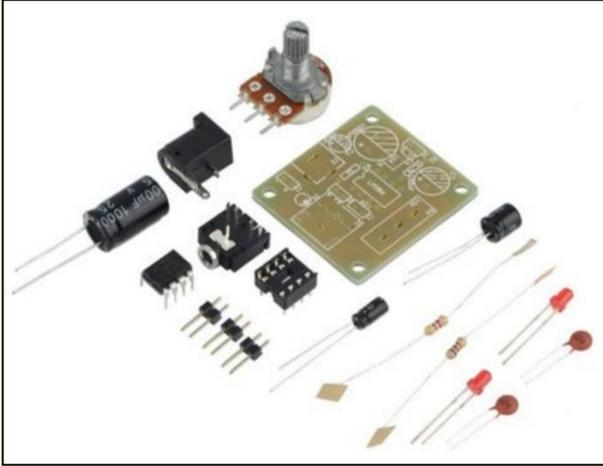
Figure 5. LM386 audio amplifier kit as ordered from eBay for less than \$2. This kit is very simple to solder together and the assembled amplifier works very well.
