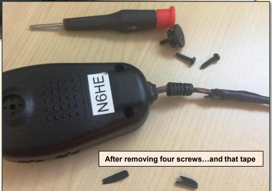
After removing four screws...and that tape
