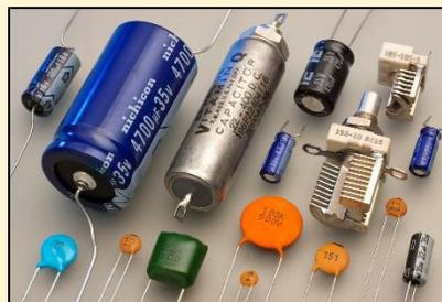
Figure 2: Examples of capacitors
