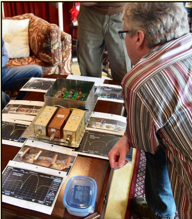
**Above:** Ron, AC6RW, examines HF triplexer developed by Jerry Kendrick, NG6R, for simultaneous 20-15-10-meter operations using three low-pass filters to enable hauling just one hexbeam antenna on our upcoming Catalina Island DXpedition.
