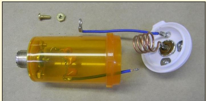
**Figure 2:** Pill bottle houses capacitors and inductor for matchbox design
