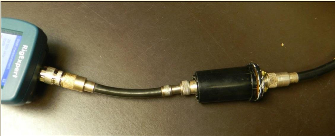
**Figure 3:** Pill bottle matchbox (prior to applying heat-shrink wrap) undergoing final testing; attached to antenna coaxial feedline on the right and to the RigExpert AA-600 antenna analyzer on the left. PHOTO: JERRY KENDRICK, NG6R
