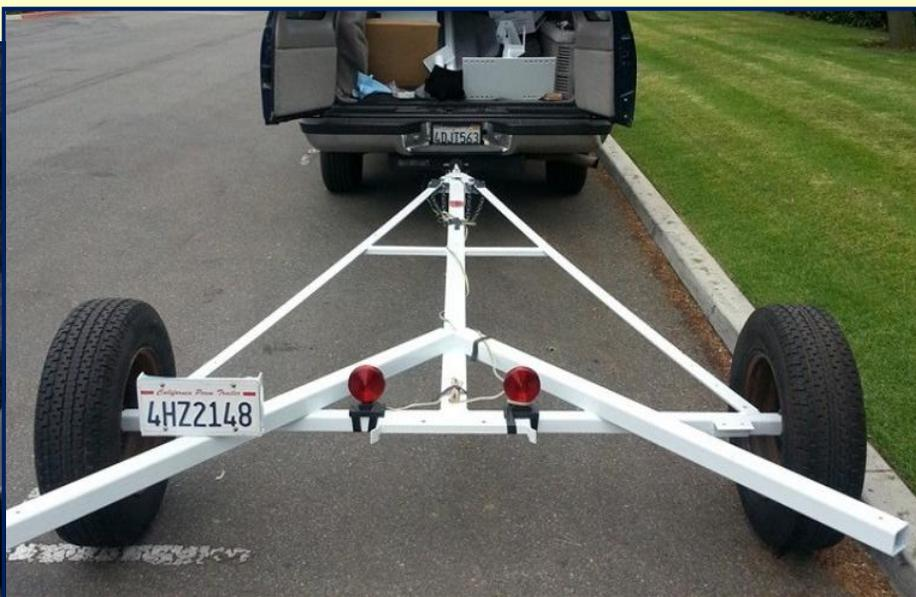
**AFTER:** Our tower trailer (with tower, structural supports, and fenders removed) in early May 2015 after being sandblasted, re-primed, and powder-coated. Joe, NZ6L, is currently re-attaching the tower and re-finished supporting elements onto the trailer, along with installing new brake light wiring to the wheel fenders. PHOTOS: JOE PACE, NZ6L
