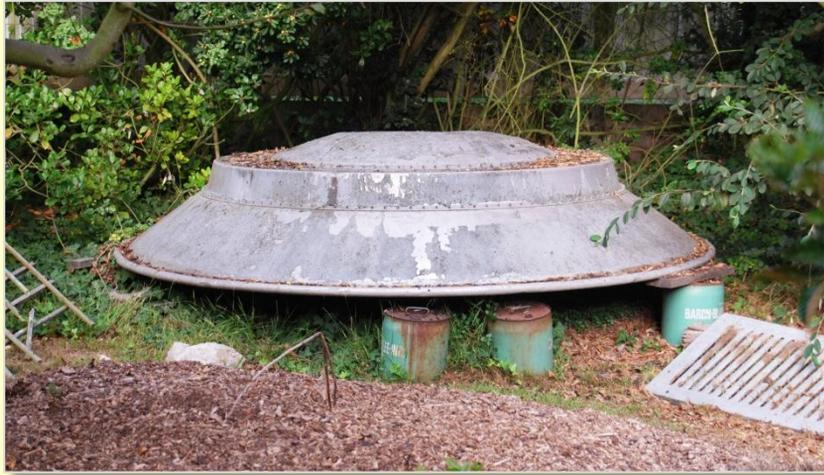
**Above:** Dish 1 is a Western Electric 3-meter diameter metal dish antenna, shown in Brian KA6UHM's backyard.
