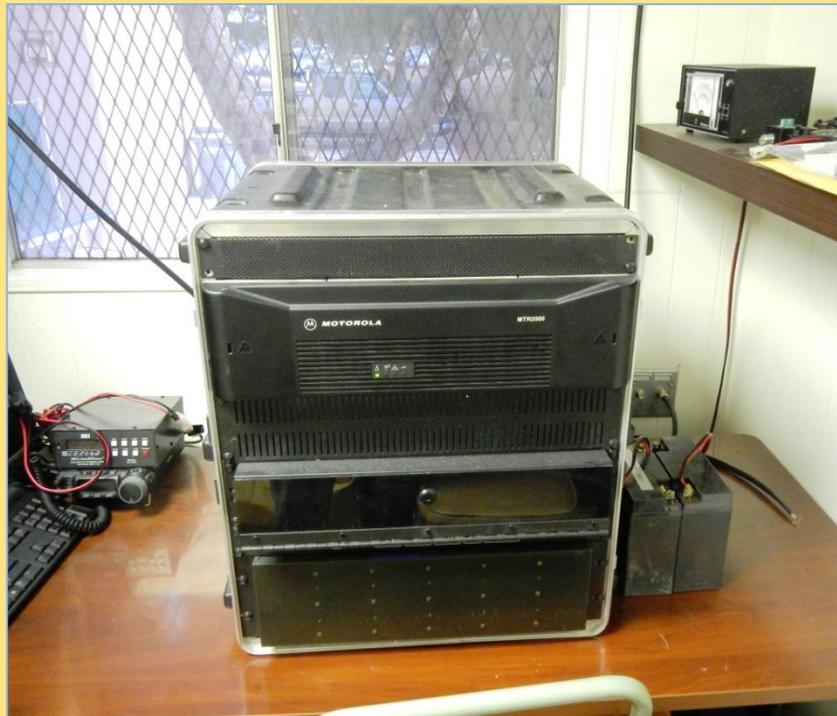
**Above:** This Motorola MTR-2000 UHF repeater loaned by Norm Thorn, K6UU, provided a hefty 50-watts for Half Marathon/10K/5K radio coverage with no worries of over-heating. Norm's repeater is rated for 100 watts continuous duty and has cavity filters plus power supply enclosed in a rugged case. PHOTO: DIANA FEINBERG, AI6DF
