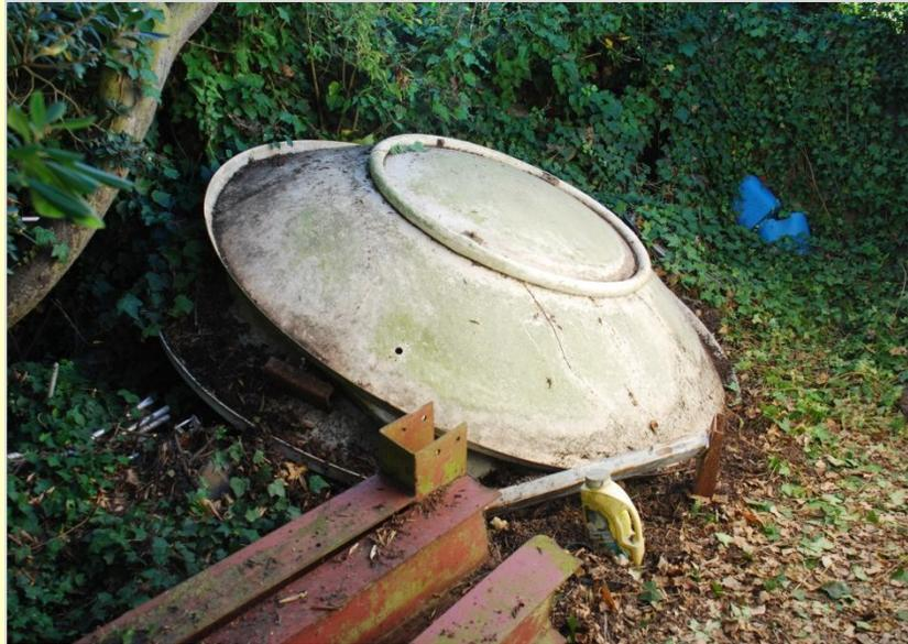
**Above:** Dish antennas 2 and 3 are made of fiberglass epoxy with an embedded metal mesh as the reflecting surface, also shown in Brian KA6UHM's backyard. The second fiberglass dish antenna is underneath the top one. Some of the angle stock that holds these dishes is shown in foreground.
