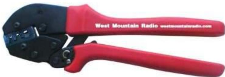
A crimper tool is used to make PowerPole connectors—no soldering required. One of these crimpers will be available to use at Elmer's Corner on November 20.
