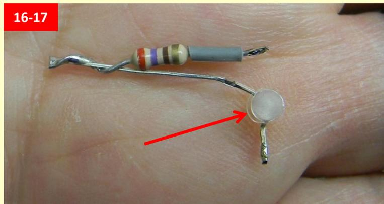
18. Heat shrink tubing is applied to the two resistor/LED combinations (white in the photo). The LEDs are inserted into the two now-vacant 3mm cavities and soldered into place. A low wattage soldering iron is highly recommended as the components are very small. Take care that each resistor is positioned so as not to interfere with any fixed PCB components when the "floating" LCD PC board is secured into place.
