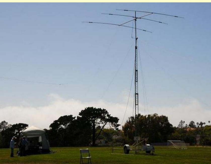
**Above:** The assembled CW antenna atop PVARC's tower trailer. PHOTO: CHRIS STOREY, KA6WNK
