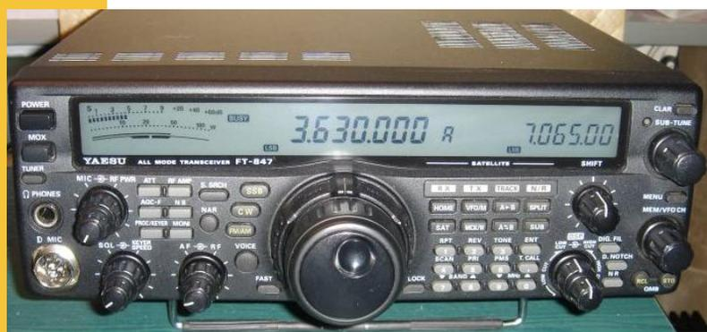
The Yaesu FT-847 multi-band transceiver, sold from 1998 through 2005, was promoted as a "satellite" radio due to its 0.1 Hz fine tuning steps for Doppler shift frequency changes; four separate antenna connections for HF, 6-meters, 2-meters, and 70-cm respectively; plus other capabilities for tracking satellites.
