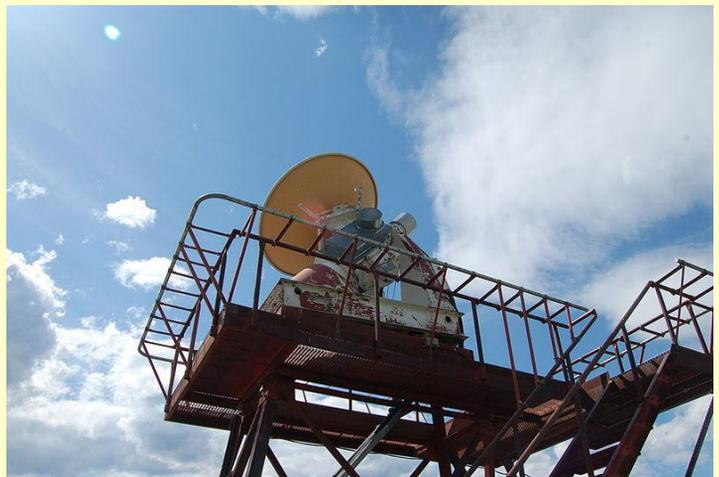
One of the two 10.7cm solar flux monitoring telescopes at the Dominion Radio Astrophysical Observatory in Penticton, BC. These telescopes provide the daily Solar Flux Index. PHOTO: JASON NISHIYAMA
