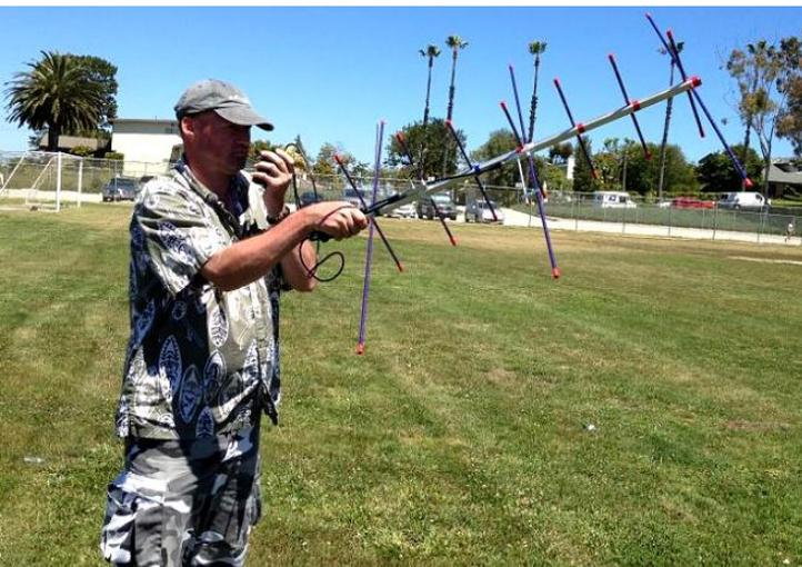
**Top left:** Rocco, N6KN, and Gary, KJ6NIY, assemble Yagi elements for CW station's tri-band beam.
