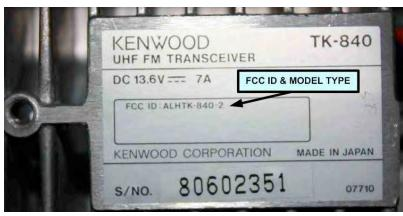
To determine the frequency range of the radio, look at the FCC ID number (Figure 2) on the back of the radio (in very small print). Typical numbers would be:
