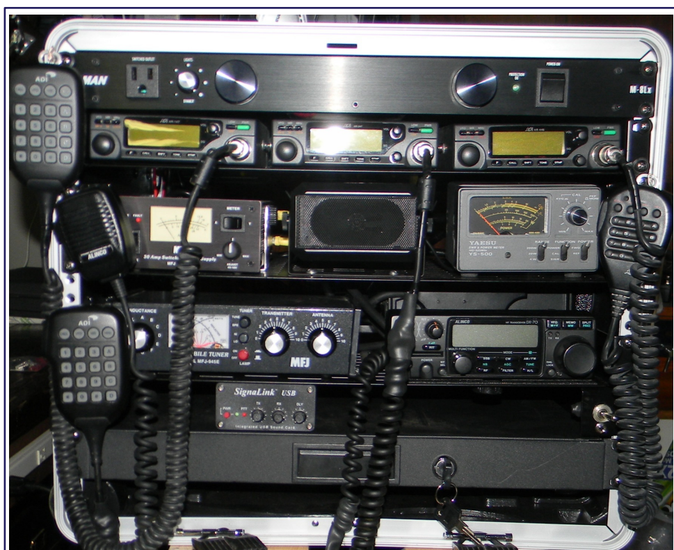
RIGHT: Our fellow member Jerry, NG6R, built this complex all-bands go-kit into an 19"-wide rack mount case.
