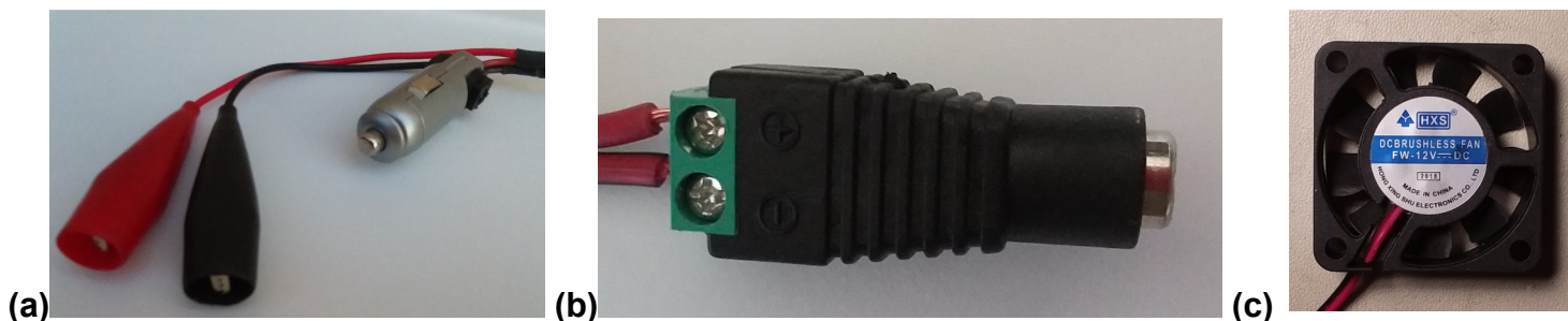
Figure 7. (a) Input DC voltage options for either automobile auxiliary power jack or battery-direct connections; (b) Universal output voltage adapter to accommodate a variety of laptop DC connector plug-ins; (c) Small and inexpensive 12VDC brushless fan to remove excess heat from enclosure. PHOTOS: JERRY KENDRICK, NG6R
