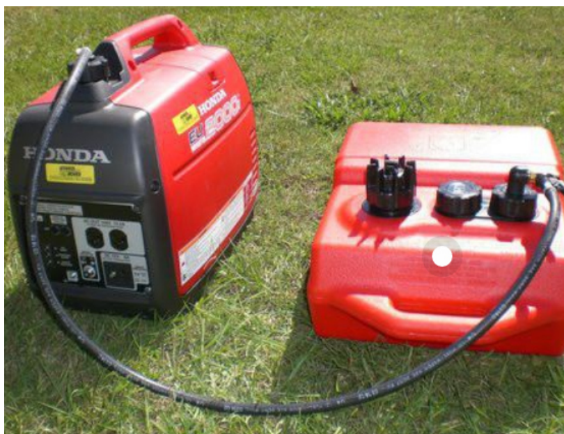
Figure 3. A portable gasoline-fueled AC generator equipped with external fuel tank for extra run time. CREDIT: https://www.pinterest.com/pin/478718635364691644/
