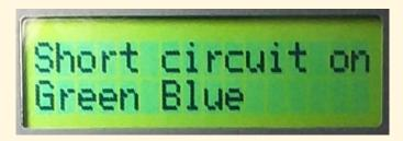
**Figure 5.** This second Mitsubishi power transistor, which failed and was replaced at the same time as example #3 above, indicates that a short exists between the collector (green) and emitter (blue). PHOTOS: JERRY KENDRICK, NG6R
