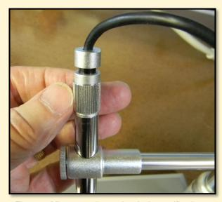
Figure 2. Microscope internal optical magnification and focus control, enabling full 2 MP of imagery PHOTO: JERRY KENDRICK. NG6R
