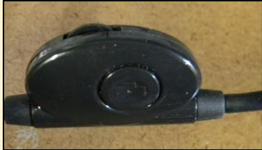
Figure 3. LED lights (*left photo*) and (*right photo*) in-line light intensity thumbwheel adjustment; snapshot pushbutton on side of control. PHOTOS: JERRY KENDRICK NG6R
